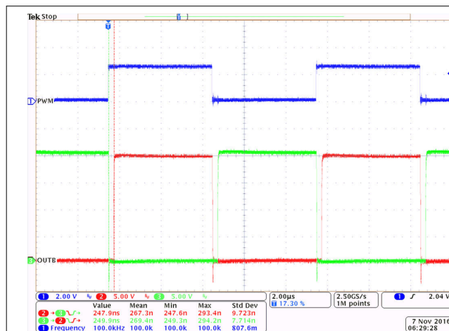
Figure 9-5. Bench Test Waveform for PWM and OUTA/B
