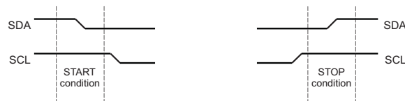
Figure 22-3. START and STOP Conditions
